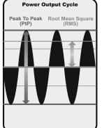
The power output is the amount of energy generated by the sonar transmitter. It is commonly measured using two methods:
